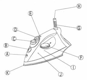
A. Spray nozzle B. Water inlet C. Variable steam control
